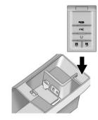
Place the new transmitter into the transmitter pocket with the buttons facing the front of the vehicle. The transmitter pocket is inside the center console storage area located between the driver and front passenger seats.
